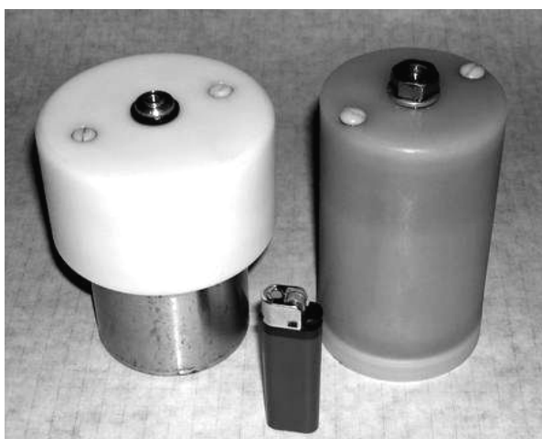
Fig. 5. External view of the peaking capacitors
