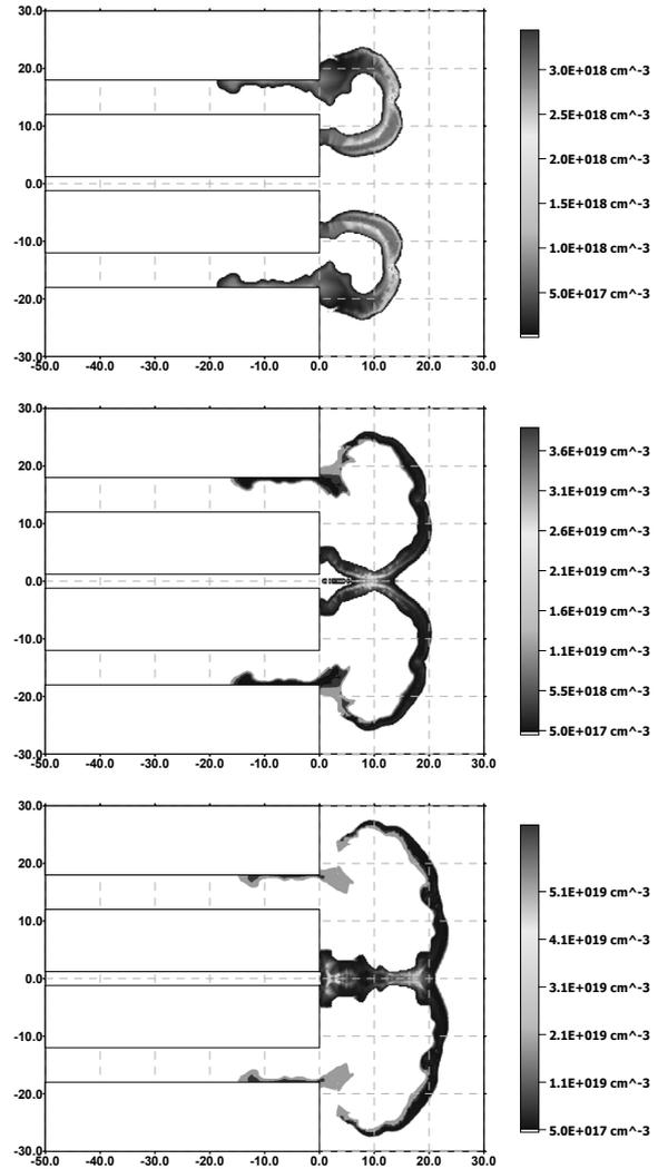
Fig. 7. Plasma density distribution during the radial collapse, as computed for the PF-1000 experiment [12] and different instants: 9  $\mu$ s, 9.7  $\mu$ s and 10  $\mu$ s after the discharge beginning
