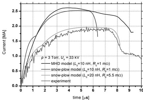
Fig. 9. Discrepancies between computed current-waveforms and experimental traces, as observed in the PF-1000 experiment [14]
