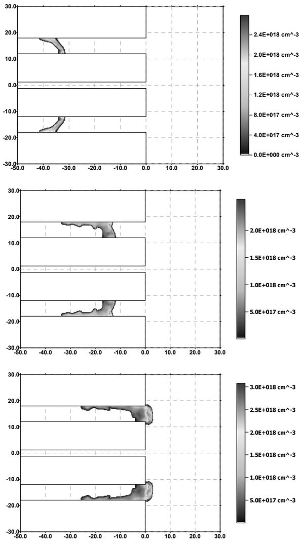
Fig. 5. Plasma density distribution in the accelerated current-sheath, as computed for the PF-1000 experiment [12] and different instants: 3  $\mu$ s, 5  $\mu$ s and 7  $\mu$ s after the discharge beginning
