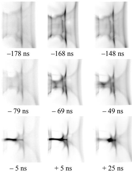
Fig. 8. High-speed frame camera pictures of the radial collapse phase, as taken in the PF-1000 experiment performed at  $p_0 = 4$  hPa,  $U_0 = 33$  kV and  $I_{\max} = 1.7$  MA (2002). Time is expressed in relation to the maximum compression
