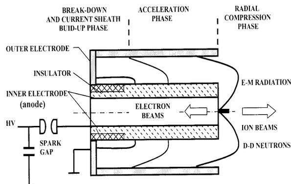
Fig. 3. Scheme of an experimental setup, showing the location of a current sheath during the three main phases of the PF-discharge
