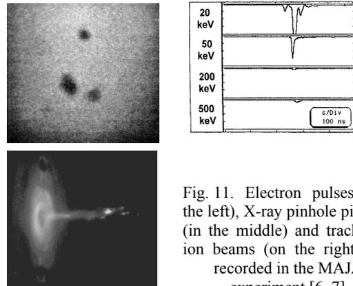
Fig. 11. Electron pulses (on the left), X-ray pinhole picture (in the middle) and tracks of ion beams (on the right), as recorded in the MAJA-PF experiment [6–7]
