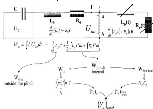
Fig. 15. Simplified PF-discharge circuit showing the parameters which determine the total neutron yield from D-D fusion reactions
