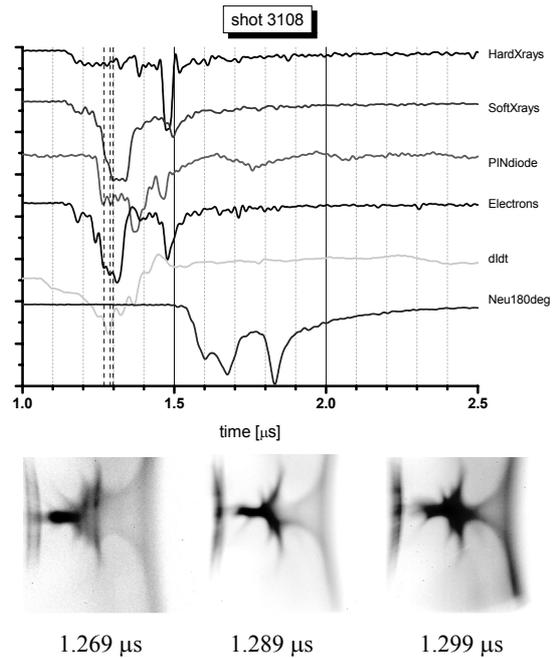
Fig. 10. Time-resolved traces and high-speed pictures of the pinch phase in the PF-1000 experiment performed at  $p_0 = 4$  hPa,  $W_0 = 734$  kJ and  $I_{\max} = 1.66$  MA [14]. The images correspond to instants indicated by broken lines
