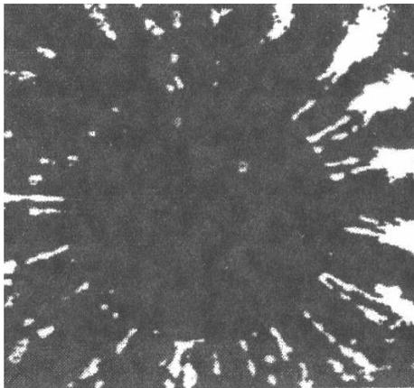
Fig. 6. Quasi-radial filaments in the CS layer during the axial acceleration, as recorded end-on with a high-speed camera [16]. A role of such filaments has not been explained so far
