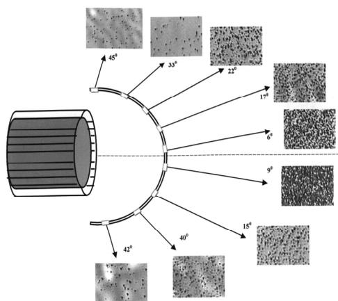
Fig.12. Ion angular distribution in the PF-1000 facility, as measured by means of NTDs placed at different angles to the z-axis [3]
