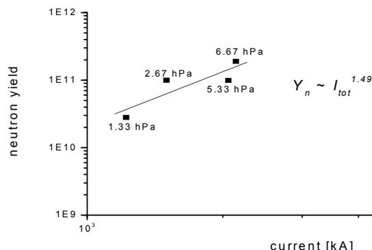
Fig.14. Neutron yield from the PF-1000 experiments performed with another set (version II) of Mather-type coaxial electrodes in order to determine the scaling law [11]
