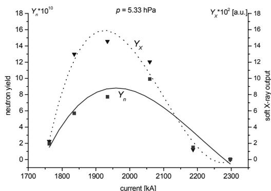
Fig.13. Neutron and X-ray yields from the preliminary experiments performed at constant initial pressure and different discharge currents in the PF-1000 machine equipped with an old set (version I) of electrodes [3]
