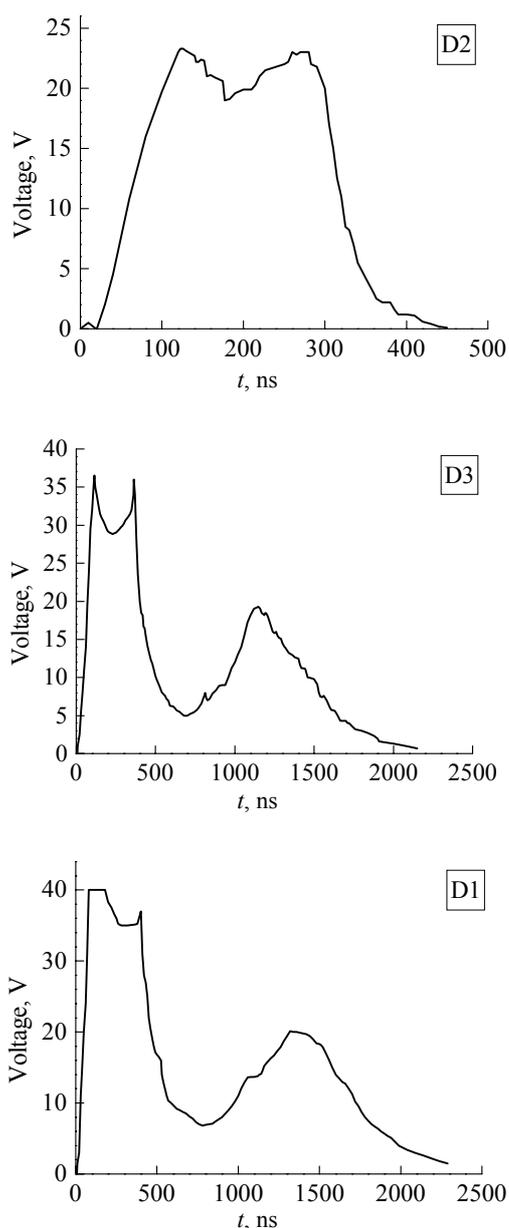
Fig. 2. Waveforms of 3 collectors located at the radii of 30 cm (D2), 129 cm (D3), and 157 cm (D1).
