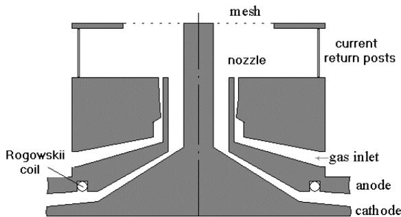
Fig. 1. Schematic of the load region
