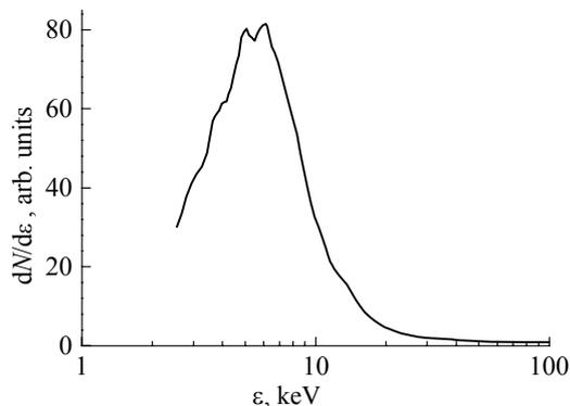
Fig. 3. Energy spectrum deduced from the D1 collector's signal (Fig. 2)
