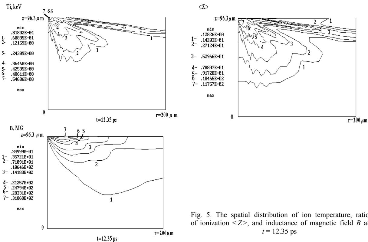
Fig. 5. The spatial distribution of ion temperature, ratio of ionization  $\langle Z \rangle$ , and inductance of magnetic field  $B$  at  $t = 12.35$  ps
