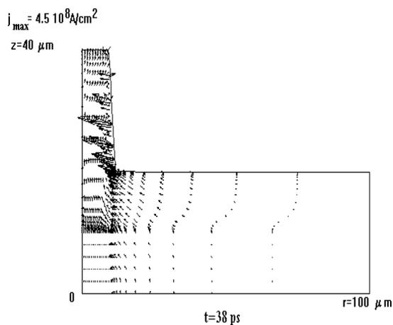
Fig. 7. The current density at  $t = 38$  ps
