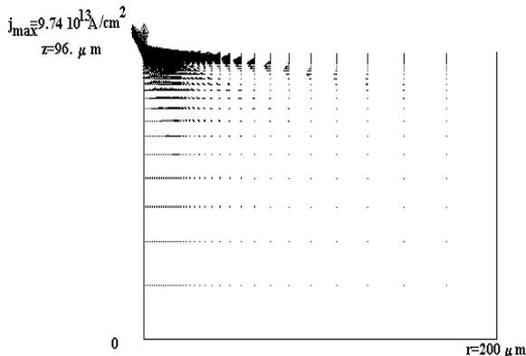
Fig. 2. The current density at  $t = 11.85$  ps
