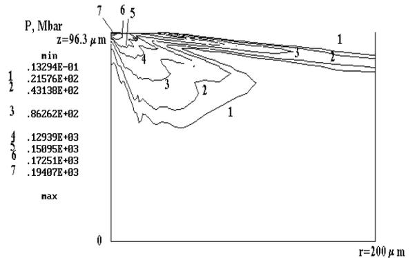
Fig. 4. The spatial distributions of total pressure in matter at  $t = 11.85, 12.35$  ps
