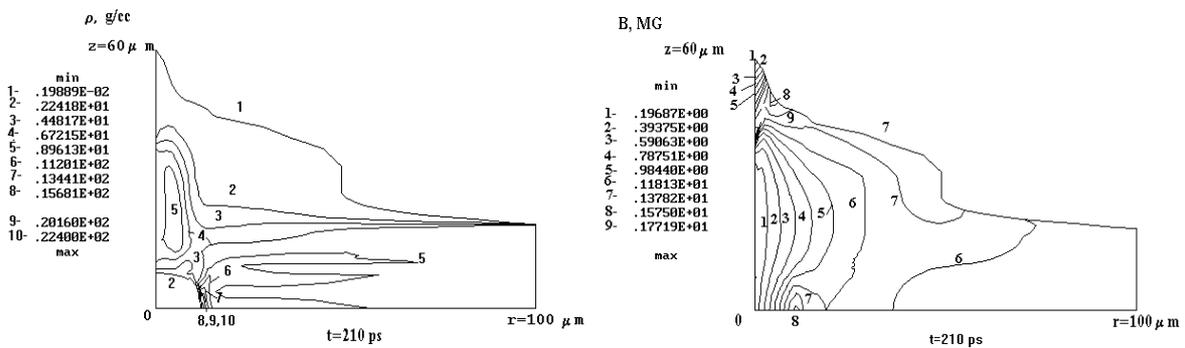
Fig. 9. The distributions of matter density  $\rho$ , inductance of magnetic field  $B$  and tension of electric field  $E$  at  $t = 210$  ps
