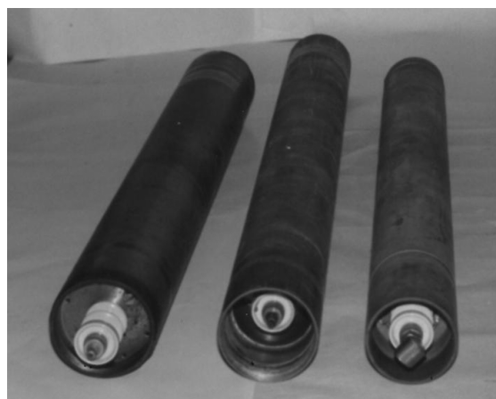
Fig. 2. High-voltage pulse capacitors for downhole devices
