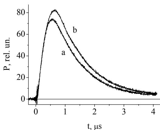
Fig. 3. Radiation power of the Xe flash lamp: *a* – mode 3; *b* – mode 2
