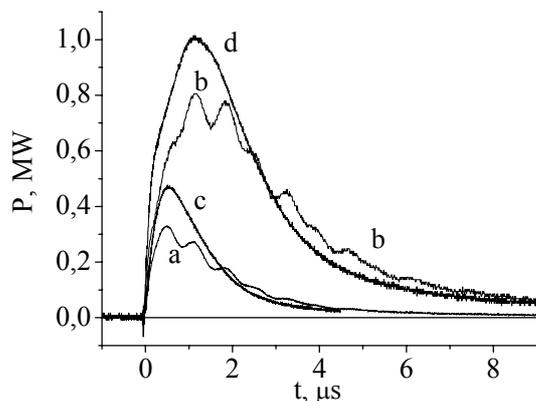
Fig. 2. Radiation power of the Xe flash lamp,  $C_0 = 260$  nF: *a*, *b* – mode 1; *c*, *d* – mode 3; *a*, *c* –  $U_0 = 9.5$  kV; *b*, *d* –  $U_0 = 24$  kV
