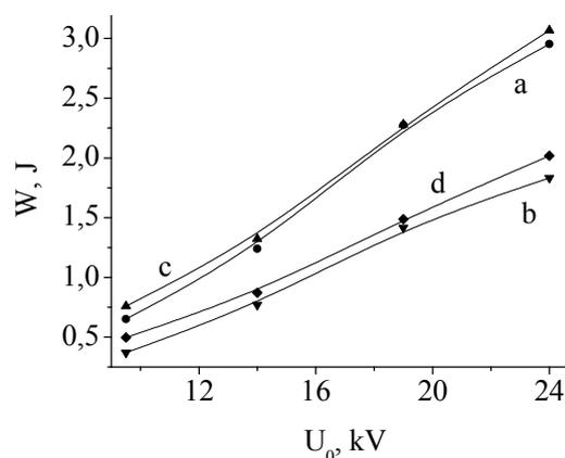
Fig. 4. The radiation pulse energy as a function of charging voltage: *a*, *b* – mode 1; *c*, *d* – mode 3; *a*, *c* –  $\lambda = 200$ –650 nm; *b*, *d* –  $\lambda = 200$ –350 nm
