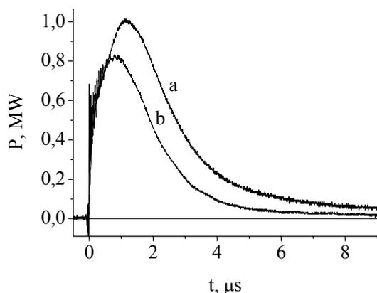
Fig. 5. Xe flash lamp radiation power measured with: *a* – FEK-22 SPU photocell ( $\lambda = 200\text{--}650$  nm); *b* – diamond detector ( $\lambda = 200\text{--}350$  nm)
