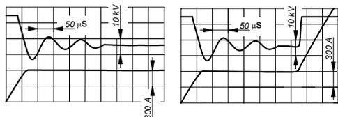
Fig. 3. The TRV oscillogram (top beam) and the breaking current oscillogram (bottom beam) (on the left – successful breaking, on the right – unsuccessful breaking)
