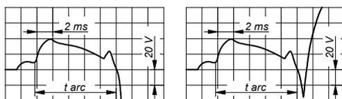
Fig. 4. The voltage oscillograms of the contacts of the interrupter (on the left – successful breaking; on the right – unsuccessful breaking)
