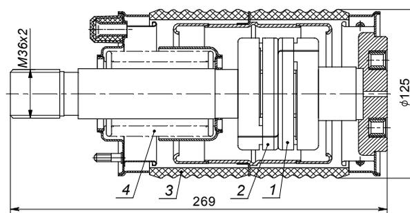
Fig. 5. A construction schematic of the vacuum arc interrupter of the KDVX4-10-40/3150 type
