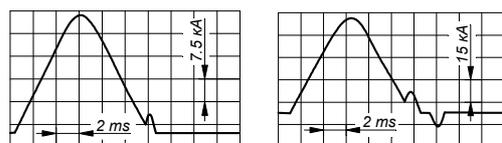
Fig. 2. Oscillograms off the current passing through the QF5 circuit-breaker being tested (on the left – successful breaking, on the right – unsuccessful one)
