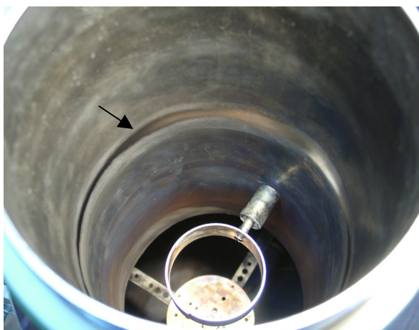
Fig. 2. Photo of the breakdown trace (melted shoulder marked by arrow) from the cathode to the wall of electron gun (after 300 shots). Diaphragms № 1 and № 2 were absent
