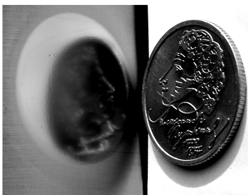
Fig. 6. Trace of the beam on the Ti surface
