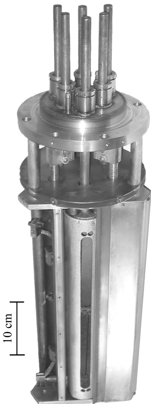
Fig. 2. Photo of the plasma generator
