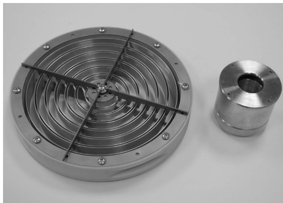
Fig. 2. Gating plate array (left) and magnetically insulated Faraday cup (right)
