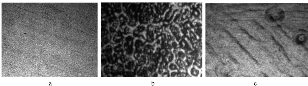
Fig. 1. Surface morphology of: (a) the unirradiated samples and the irradiated by one pulse with average ion current density 150 (b), 10 (c) A/cm<sup>2</sup> ( $\times 200$ )
