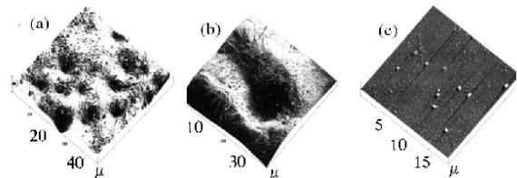
Fig. 4. Craters with internal string structure(a); a large cumulative crater (b); side of a silicon target with cumulative nano-particles of vanadium (c)
