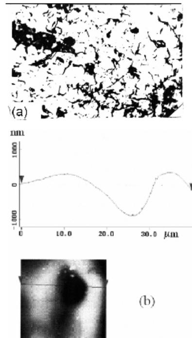
Fig. 3. The surface of a plate of vanadium with thickness of 0.22 mm – the side opposite the irradiation (a); the shock crater with rim (b)
