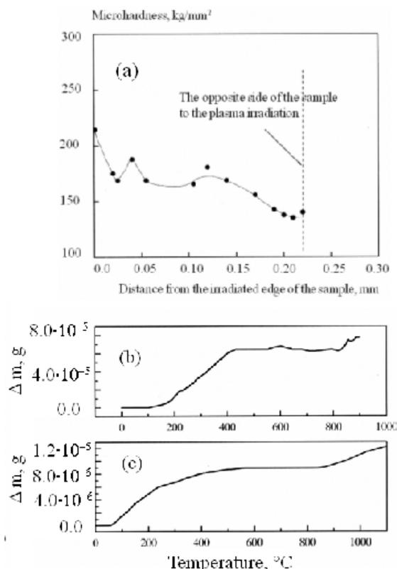
Fig. 2. Change of microhardness on a cross-section of the irradiated sample of vanadium (a); change of weight of the irradiated sample of vanadium at an isochronal annealing up to 900 °C (the first annealing) (b); change of weight at the repeated annealing (c)
