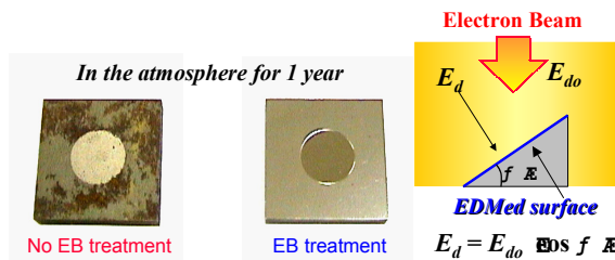
Fig. 7. Comparison of corrosion in the atmosphere for 1 year
