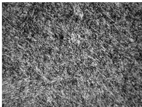
Fig. 1. Microstructure of high-strength steel ( \times 1000 )
