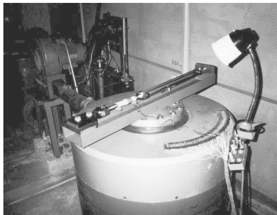
Fig. 3. Outward appearance of plant for specimen fretting testing (on the basis of ВЭДС-1500 vibrobed)
