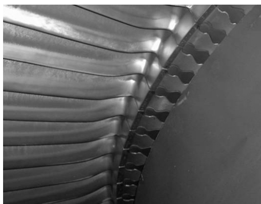
Fig. 7. Shank view of CLP blades of PS "Alholma" turbine after 13 388 operating hours
