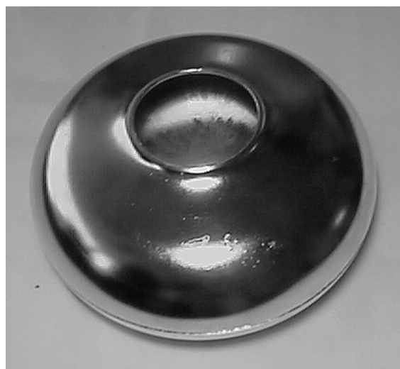
Fig. 2. TESLA type copper cavity, which was coated with a pure Nb layer at IPJ in Swierk
