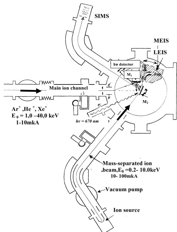
Fig. 3. Scheme of the analytical chamber with two ion beams and different diagnostics tools,  $M_1$  and  $M_2$  are targets for sputtering and deposition
