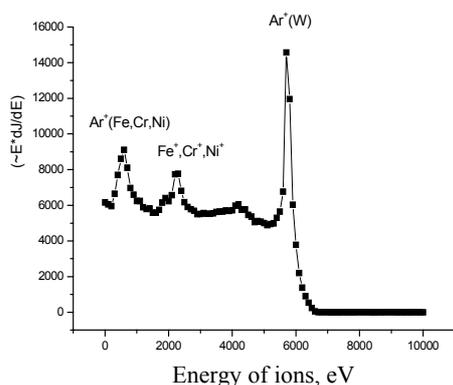
Fig. 4. Energy spectra of ions scattered and knocked out from the stainless steel target after deposition by reactive sputtering of tungsten atoms detected by energy analyzer during sputtering of stainless steel target (substrate target) after reactive deposition on it (at temperature ~600 °C) of several monolayers of tungsten
