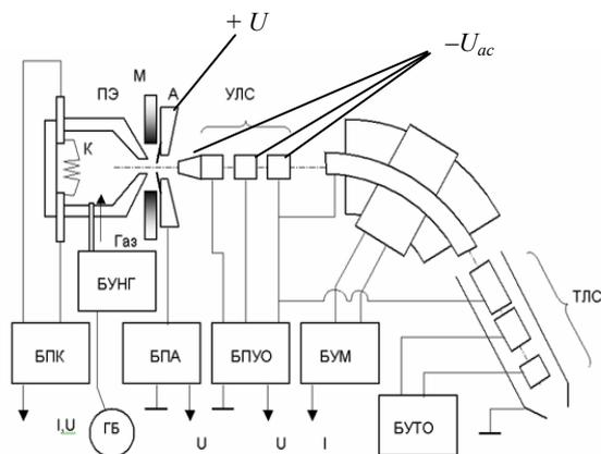
Fig. 1. Scheme and power supply of the low energy ion channel: УЛС – accelerating and focusing system, БПК – cathode supply, БУНГ – gas feed system, БПА – anode supply, БПУО – supply of accelerating optics, БУМ – electromagnet supply, БУТО – retarding system control, ТЛС – retarding lens system
