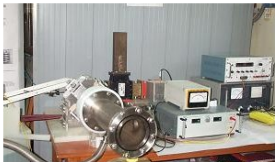
Fig. 2. E.C.R Ion source
