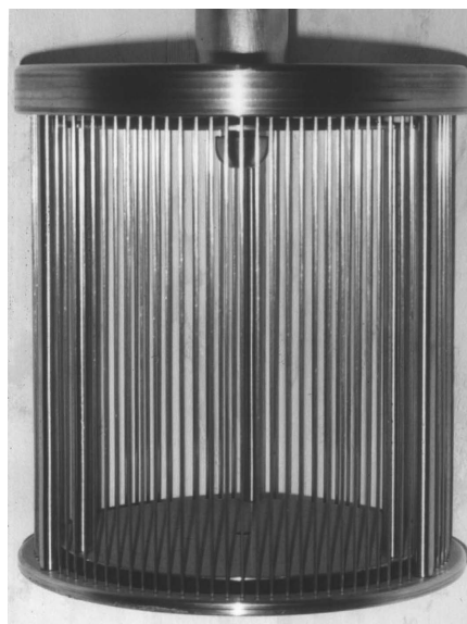
Fig. 7. Beam source with a cylindrical 20-cm-diam and 20-cm-high grid made of parallel 1.5-mm-diam steel wires
