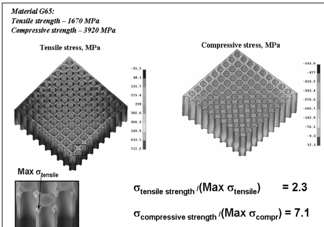
Fig. 1. Finite element analysis of honeycomb die made of WC-Co. Tensile strength and compressive strength both are higher than the stresses calculated by finite element method
