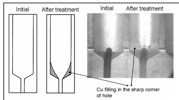
Fig. 2. After EB melting, some accumulations of Cu remain in the sharp corner of the hole. It may provide a streamlined shape which can perform laminar flow during SiC extrusion
