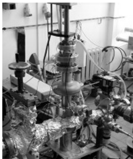
Fig. 2. UHV system with a linear-arc and a TESLA-type RF cavity, as shown during tests in Swierk
