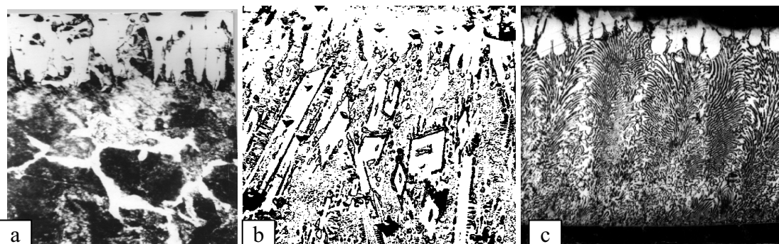
Fig. 1. Layers boride microstructure formed on steel 45 surface: solid phase borating (a) and electron beam boriding – daub from amorphous boron (b) and B_4C (c); a – 250, b, c – 500
