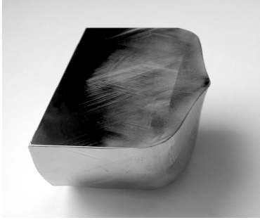
Fig. 1. Light microscope image of dislocated FZ-Si ingot etched in (110) cross-section by a selective chemical etchant.
