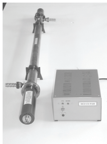
Fig. 4. Photochemical reactor with a power supply on the basis of the one-barrier Xe-excimer lamp
