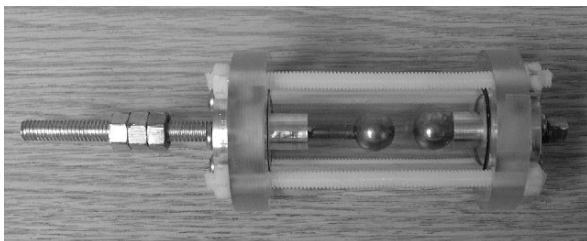
Fig. 3. Spark gap assembly for HV holdoff tests
