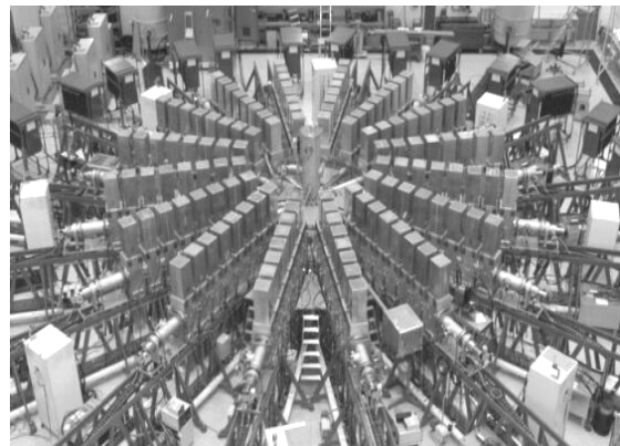
Fig. 1 Sphinx machine, 16m diameter, 3m height 16 branches, 8 LTD-05 stages per branch
